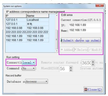
C. Set the IP address as the default Localhost Link1 communication port is selected to correspond to the PLC download line of the authorization code computer.
