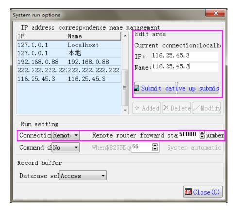
E. Set the IP address as the default Localhost Link1 communication port to be selected as the PLC download line of the authorization code computer.
