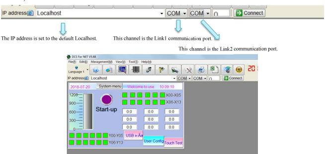
Connect the computer to the PLC using the PLC download line. The COM port corresponding to the PLC download line is COM3:
