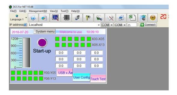
The COM port corresponding to the PLC download line of the authorization code computer is set to COM3:
